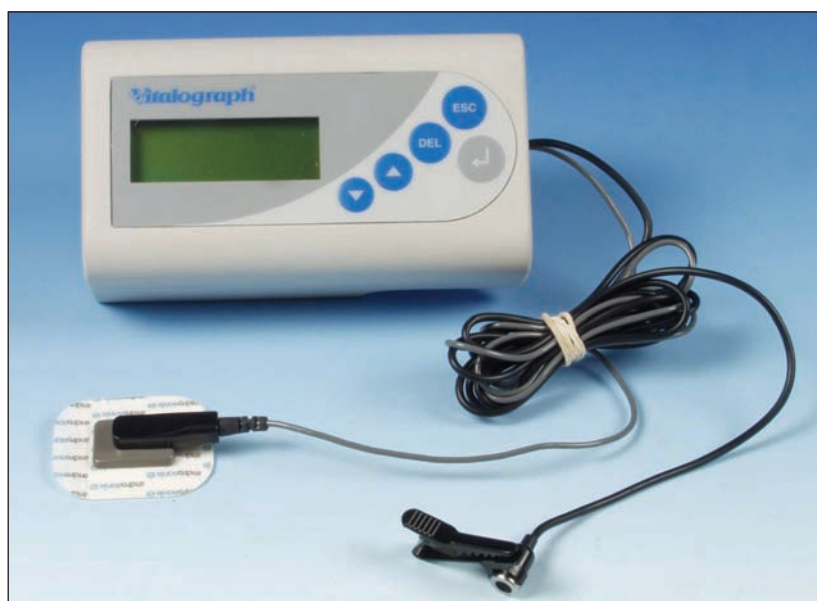
Figure 6: VitaloJAK cough monitoring device.
